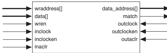
Figure 23. APEX 20KE CAM Block Diagram
