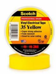
Scotch® Vinyl Electrical Tape 35 is a 7-mil thick, premium-grade, color-coded electrical tape. This flame-retardant tape is suitable for use in phase identification, color coding of motor leads and piping systems and for marking safety areas. This tape is 600V-rated and withstands a temperature range of 32 to 221 degrees F (0 to 105 degrees C).
