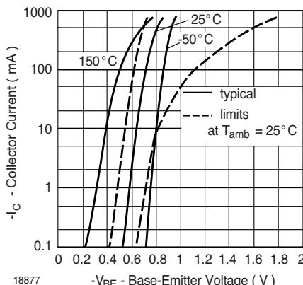
Fig. 3 Collector Current vs. Base-Emitter Voltage
