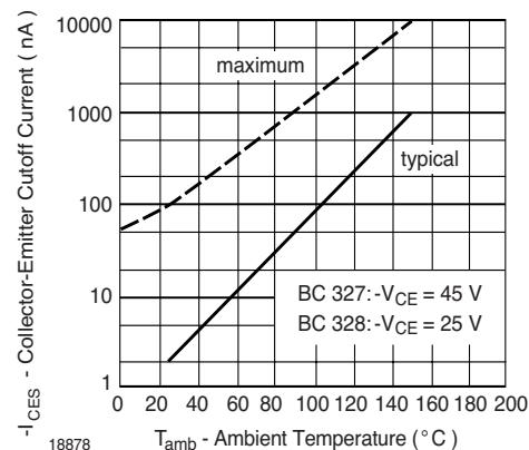
Fig. 4 Collector-Emitter Cutoff Current vs. Ambient Temperature
