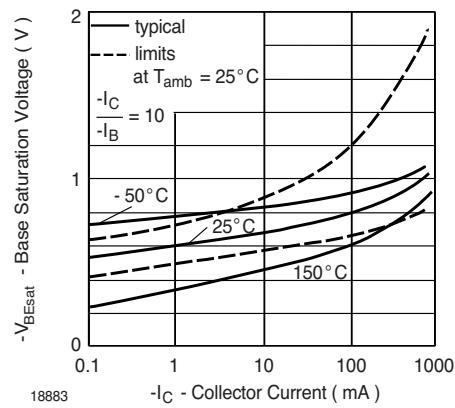
Fig. 10 Base Saturation Voltage vs. Collector Current
