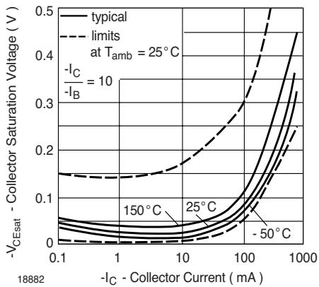
Fig. 9 Collector Saturation Voltage vs. Collector Current
