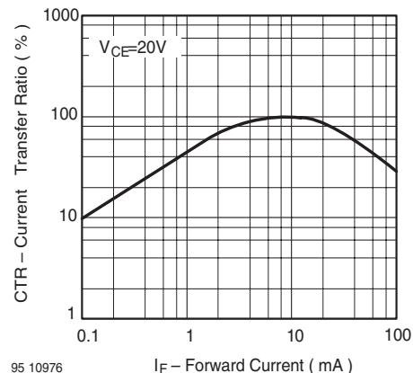
Figure 15. Current Transfer Ratio vs. Forward Current
