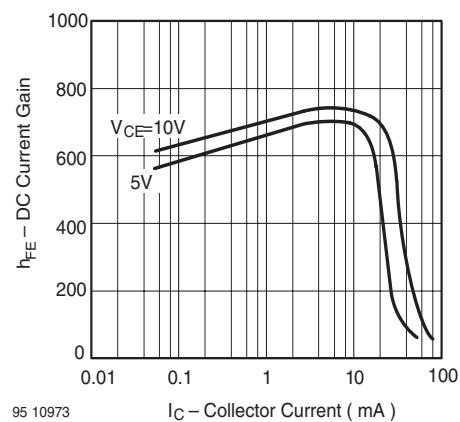
Figure 14. DC Current Gain vs. Collector Current
