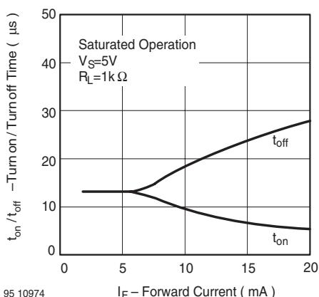
Figure 16. Turn on / off Time vs. Forward Current
