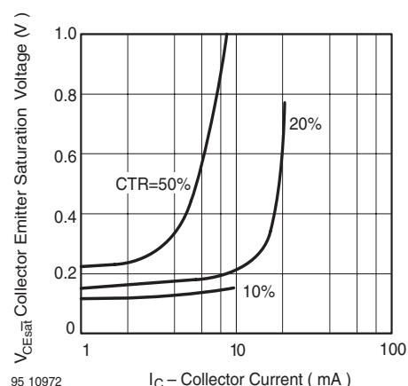
Figure 13. Collector Emitter Saturation Voltage vs. Collector Current
