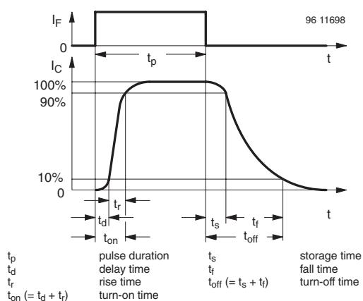
Figure 5. Switching times
