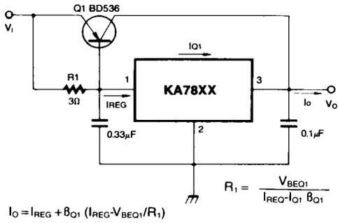
Fig. 13 High Output Current with
