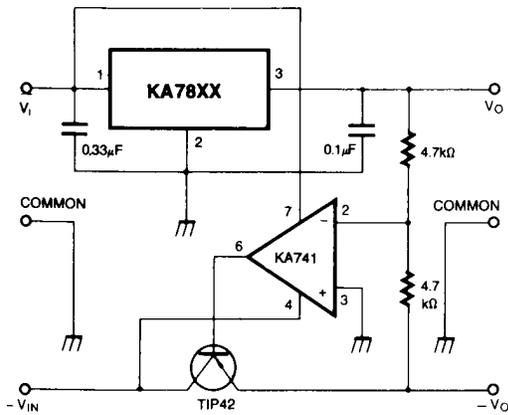
Fig. 15 Split Power Supply (±15V-1A)
