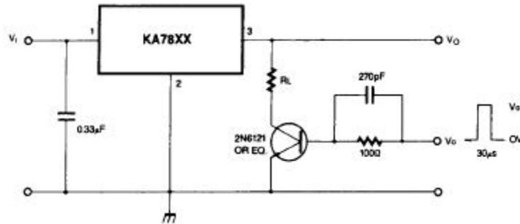
Fig. 7 Ripple Rejection
