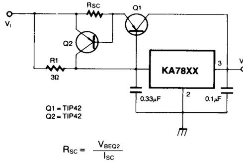
Fig. 14 Tracking Voltage Regulator
