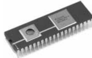
Ceramic Sidebrazed Dual-in-Line Package Product Suffix: D
