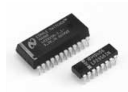
Molded Dual-in-Line Package (DIP) Product Suffix: N
