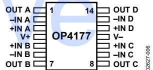
Figure 6. 14-Lead TSSOP (RU Suffix)
