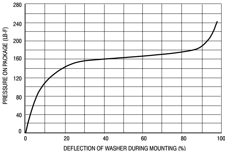
Figure 5-9. Characteristics of the Conical Compression Washers Designed for Use with Plastic Body Mounted Semiconductors
