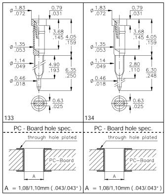
E-tec offers solid press fit sockets in any standard pin-out and with 2,54mm/.100" pitch.
