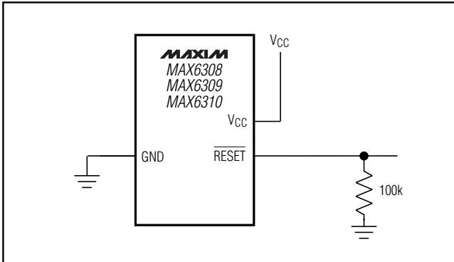
Figure 4. Ensuring  $\overline{\text{RESET}}$  Valid to  $V_{CC} = 0\text{V}$
