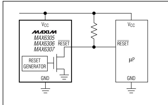
Figure 3. Interfacing to μPs with Bidirectional Reset I/O
