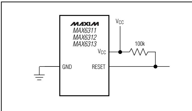
Figure 5. Ensuring  $\overline{\text{RESET}}$  Valid to  $V_{CC} = 0\text{V}$
