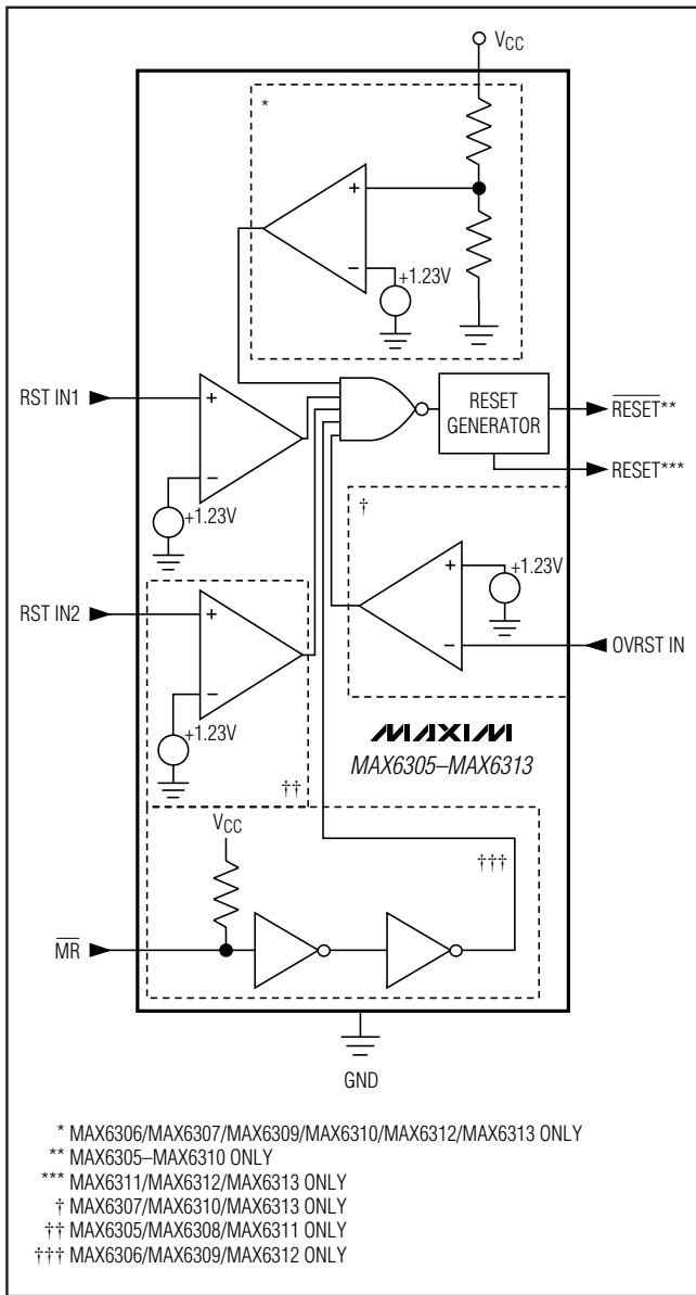
Figure 1. Functional Diagram
