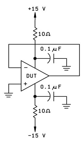
FIGURE 2. Radiation exposure circuit.
