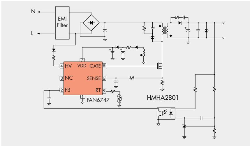
Isolating Feedback Loop to Highly Integrated Green-Mode PWM Controller
