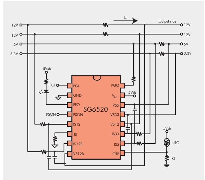
SG6520: Typical Application Circuit with Minimal External Components
