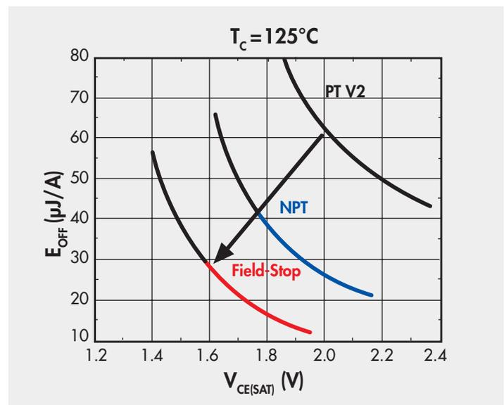
600V IGBT Trade-off Curve ( $E_{OFF}$  vs.  $V_{CE(SAT)}$ )
