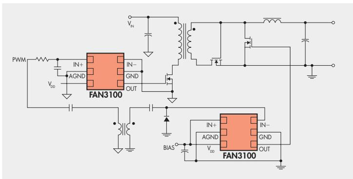
Forward Converter with Hybrid Synchronous Rectifier
