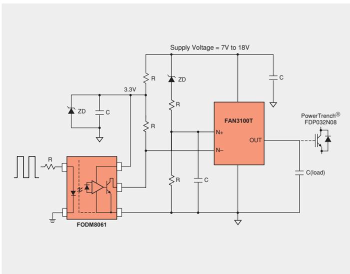
*High-Speed Optocoupler drives the Low-Side Gate Driver for IGBT Control*
