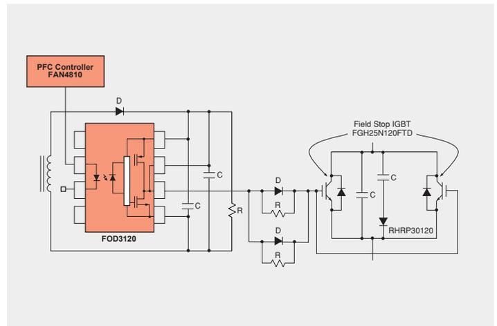
Optically Isolating the PFC Controller and the IGBTs
