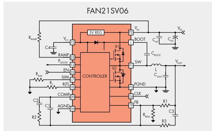
Fully Integrated Synchronous Buck Regulator Featuring External Synchronization and Internal 5V Regulator
