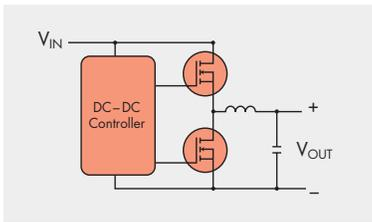
Synchronous Buck for DC-DC Applications
