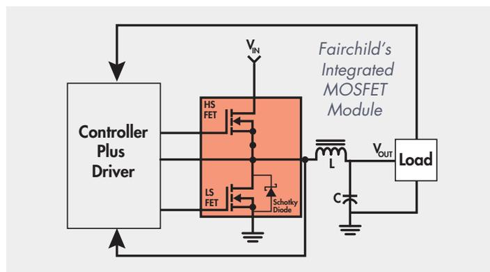
Buck Converter Block Diagram
