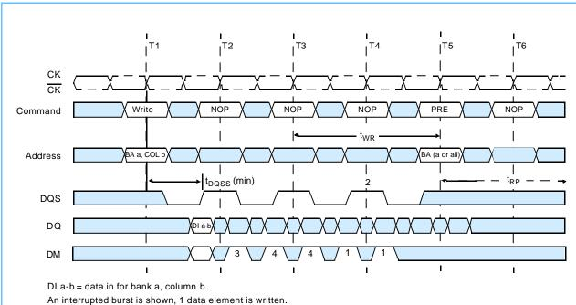
$t_{\mbox{\scriptsize WR}}$  is referenced from the first positive CK edge after the last desired data in pair.
