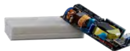
Infineon's 20 W/in 3 adapter (cased) - 24 W/in 3 (uncased) with 65 W output power capability (LxWxH: 74.2 mm x 36.5 mm x 16.5 mm)
