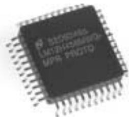
Ceramic Quad Flatpack (Gullwing) Product Suffix: WG
