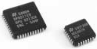
Molded Plastic Leaded Chip Carrier (PLCC)
