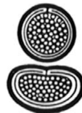
Strands enter as a homogeneous group and compact tightly under compression due to fully brazed seam
