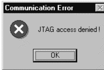
Figure 2–3. Communication Error Box for Blown Fuse
