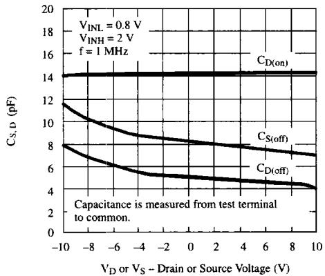
**Capacitance vs. VD or VS (DG186)**
