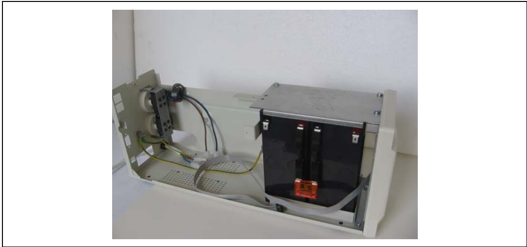
Figure 32. UPS with AVR transformer
