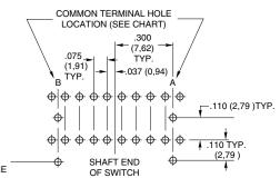
Shown for a two deck switch. Bushing mount is recommended.
