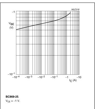
Fig.10 Base-emitter voltage as function of collector current; typical values.
