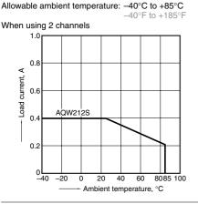
1.-(2) Load current vs. ambient temperature characteristics Allowable ambient temperature:  $-40^{\circ}$ C to  $+85^{\circ}$ C
