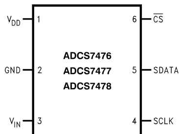
Figure 1. 6-Lead SOT-23 or WSON See DBV or NGF Package
