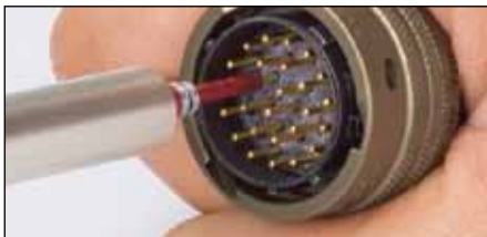
Typical application showing tool testing pin contacts.
