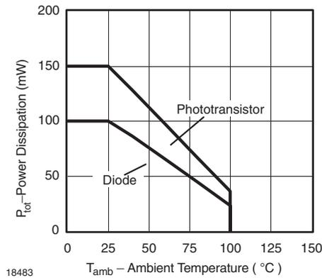
Figure 1. Permissible Power Dissipation vs. Ambient Temperature
