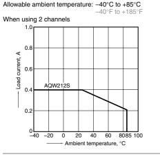
1.-(2) Load current vs. ambient temperature characteristics
