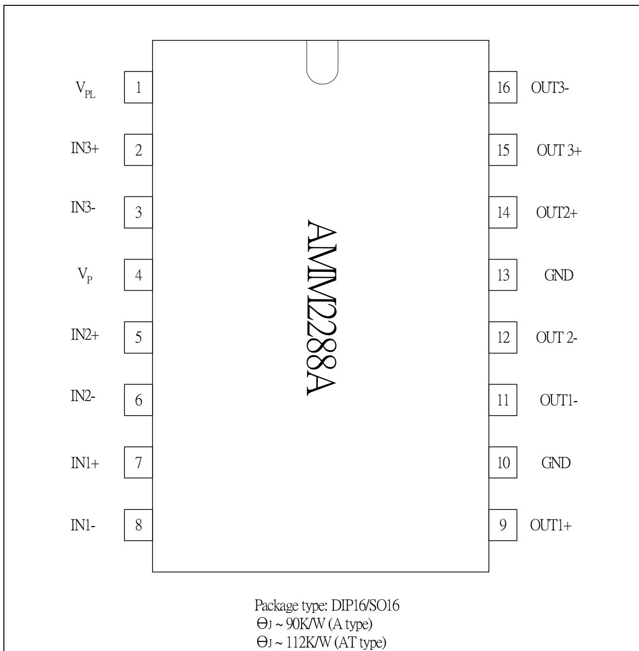
The AMM2288 is triple power driver circuits in a BTL configuration, intended for use as a power driver for servo systems with a single supply. It is particularly designed for **compact disc players** and is capable of driving focus, tracking, sled , spindle functions and loading motors.
