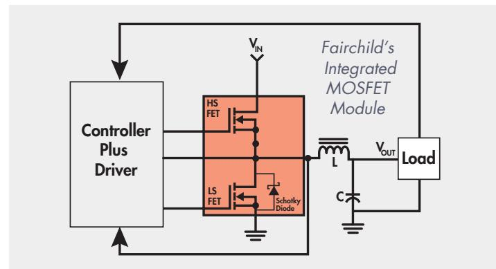
Buck Converter Block Diagram
