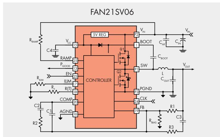
Fully Integrated Synchronous Buck Regulator Featuring External Synchronization and Internal 5V Regulator
