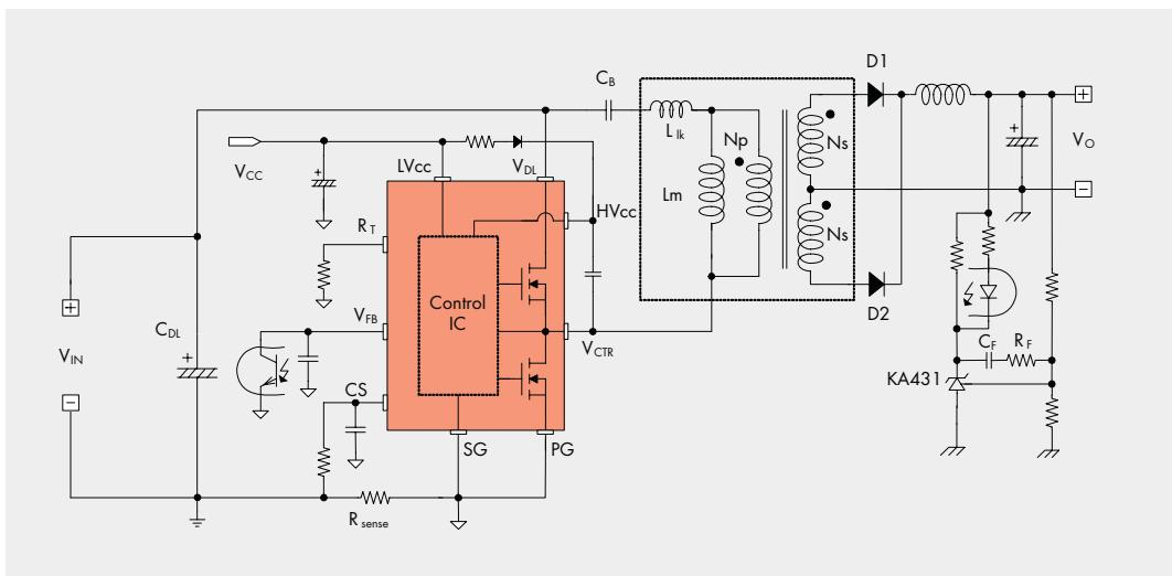
Typical Application Circuit for an Asymmetric PWM Half-Bridge Converter
