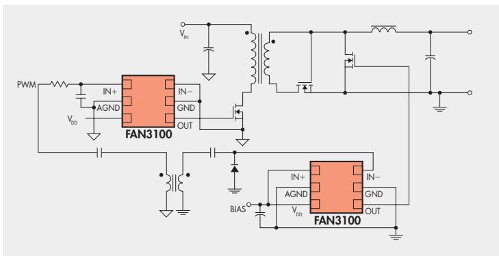
Forward Converter with Hybrid Synchronous Rectifier
