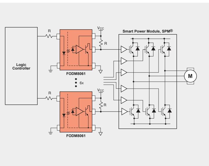
High-Speed Optocoupler drives Intelligent Power Module to prevent catastrophic failure of the motor drive, and meet safety regulatory standards
