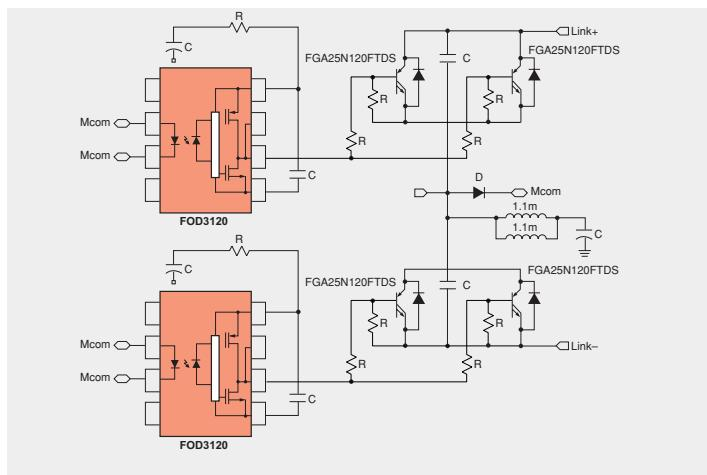
*Optically Isolating the Inverter Output within the UPS*
