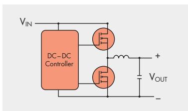
Synchronous Buck for DC-DC Applications
