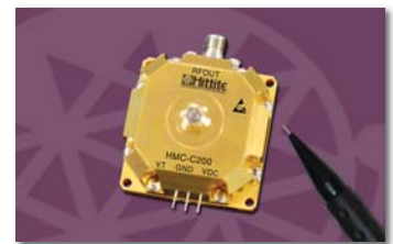
HMC-C200 Dielectric Resonator Oscillator (DRO) Module.
