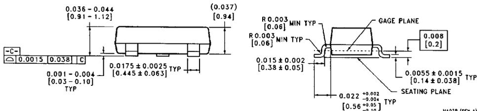
SOT-23 Molded Small Outline Transistor Package (M3)
