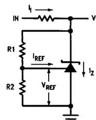
Note:  $V_Z = V_{REF} (1 + R_1/R_2) + I_{REF} \cdot R_1$
