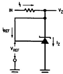
FIGURE 1. Test Circuit for  $V_Z = V_{REF}$
