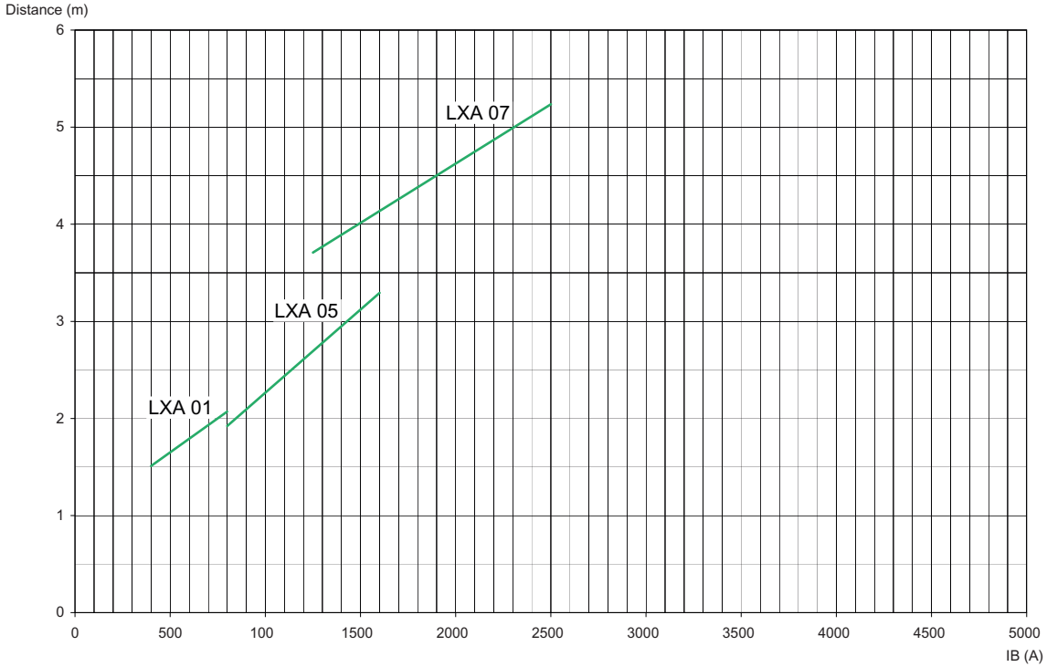
Figure 7-15 LXA load distance profile for 0.2 \mu\text{T} of systems 800 A, 1600 A and 2500 A
